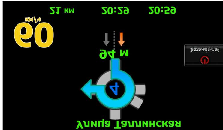
In the skin and its modes added support **Head-Up Display (HUD)** – Mirror Display: navigation information is projected directly into the line of sight on the windshield.
