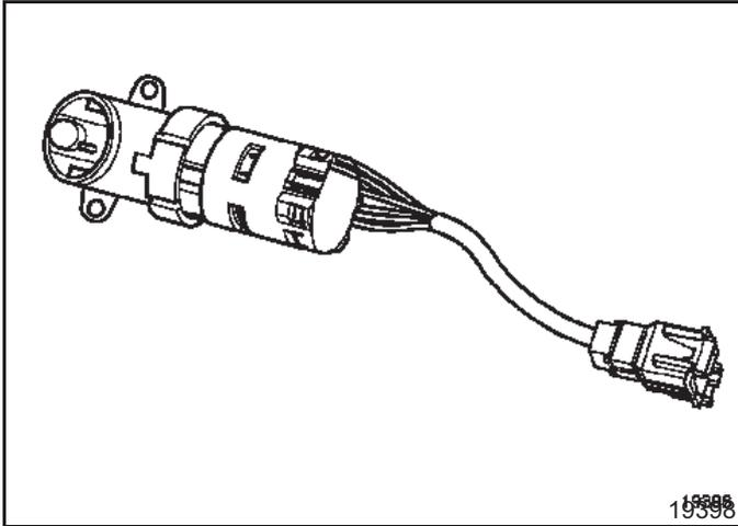
The sensor measures the humidity in the passenger compartment.
